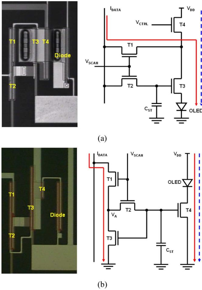
Fig. 5. Top view of fabricated (a) conventional current-driven and (b) current-mirror pixel-electrode circuits based on a-Si:H TFTs.
