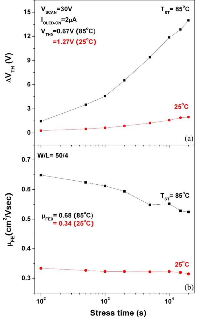
Fig. 9. Variations of threshold voltage and field-effect mobility of a-Si:H TFT ( $W/L = 50/4$ ) as a function of stress time at  $25^\circ C$  and  $85^\circ C$ .
