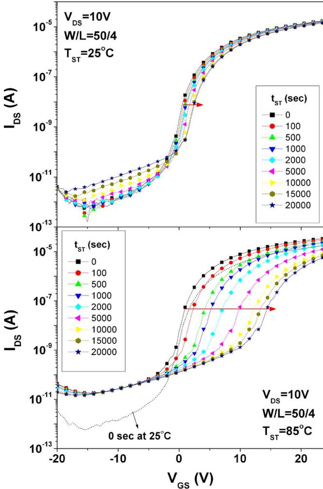
Fig. 8. Transfer characteristic of TFT ( $W/L = 50/4$ ) after current-stress ( $I_{DATA} = 2 \mu A$ ) as a function of stress time (a) at room temperature ( $25^\circ C$ ) and (b) at  $85^\circ C$ .
